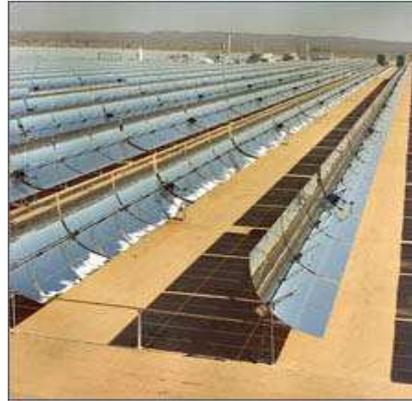
Many power plants today use fossil fuels as a heat source to boil water. The steam from the boiling water spins a large turbine, which drives a generator to produce electricity. However, a new generation of power plants with concentrating solar power systems uses the sun as a heat source. The three main types of concentrating solar power systems are: *linear concentrator*, *dish/engine*, and *power tower systems*.
