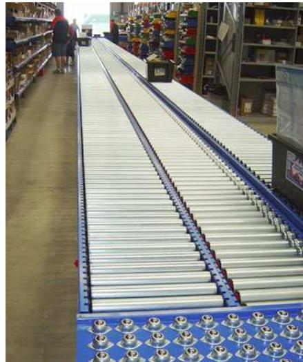
Conveyors should be appropriately guarded, including the installation of fixed guards at trapping points or, in certain cases, interlocking guards.
